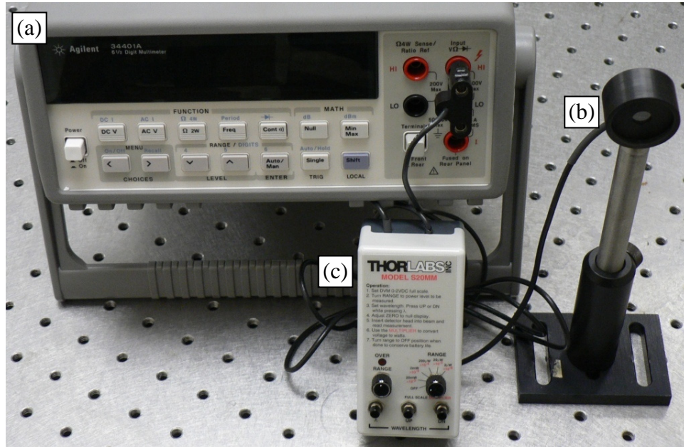
Figure 6.2: Photograph of equipment used to measure laser power. (a) The Agilent® 34401A digital multimeter displays the power values from (b) the Thorlabs® S20MM silicon power meter head and (c) the meter controller. Not shown are the absorptive neutral density filters that attach to the power meter for high-power measurements.
