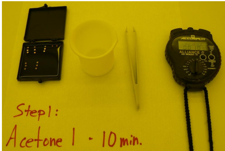
Figure 6.20: Photograph of the first step in the release process—a 10-minute acetone bath. Shown are the chips, an acid-resistant beaker, acid-resistant tweezers, a stopwatch, and a piece of labeled clean room paper. Labeling the paper helps prevent mistaking de-ionized water with HF, for example.
