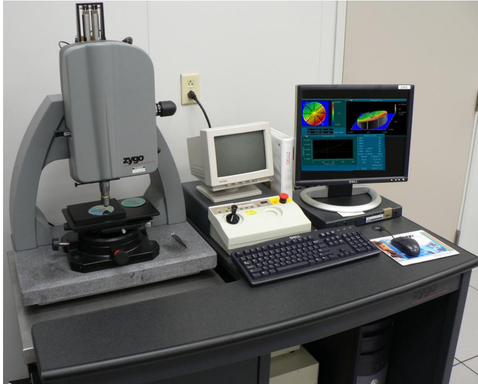
Figure 6.26: Photograph of the Zygo ® interferometric microscope workstation used to precisely measure microrobot vertical deflection.
