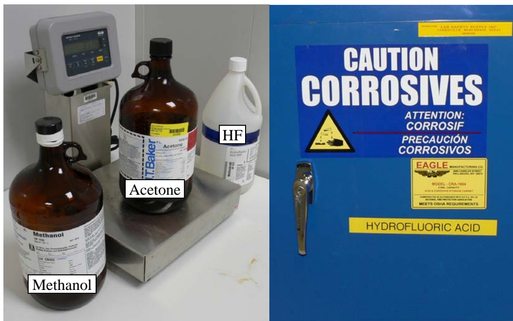
Figure 6.18: Photographs of the three chemicals used in the release procedure—methanol, acetone, and hydrofluoric acid (HF)—on a weighing scale (left) and the separate storage unit for the highly corrosive HF (right).
