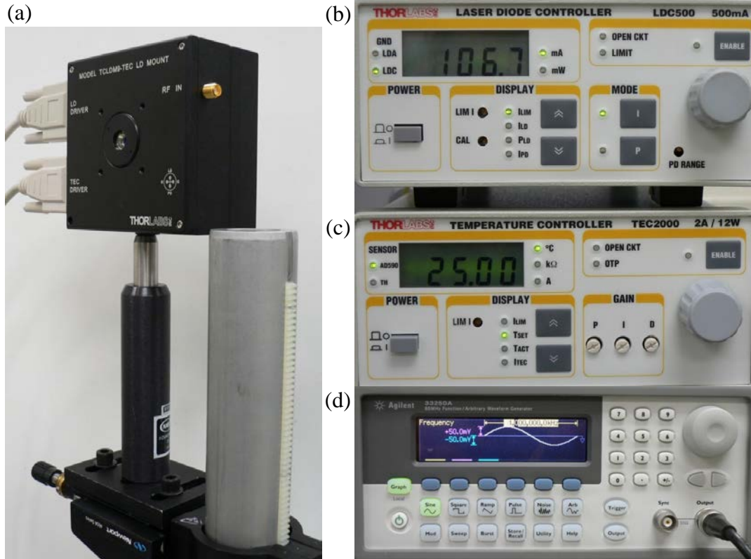
Figure 6.1: Photographs of laser operating equipment. (a) The ML101J8 laser diode is inside the TCLDJ8 diode mount; (b) the LDC 500 diode controller powers the diode; (c) the TEC 2000 temperature controller ensures the diode temperature is constant; (d) and the 33250A function generator modulates the LDC 500 controller for pulsed operation.
