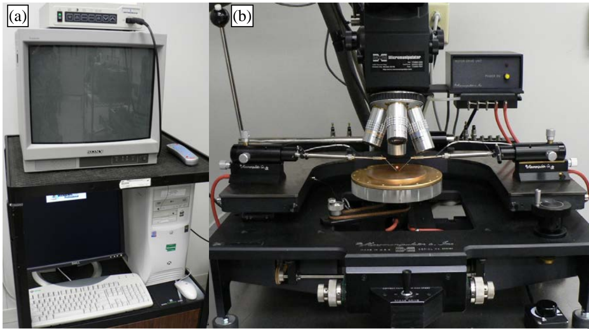
Figure 6.29: Photographs of (a) video capture equipment and (b) the Micromanipulator ® probe station used for inspecting, applying power to, and probing MEMS samples.
