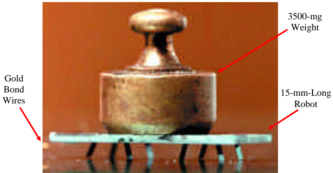
Figure 2.15: Photograph of 15-mm-long robot carrying a 2500-mg weight (30 times its own weight), which is a record for miniature robots. Note the gold bond wires supplying power on the left side of the robot. This robot set a miniature walking robot ground speed record at 12 mm/second but required 1.1 W to do so [56].
